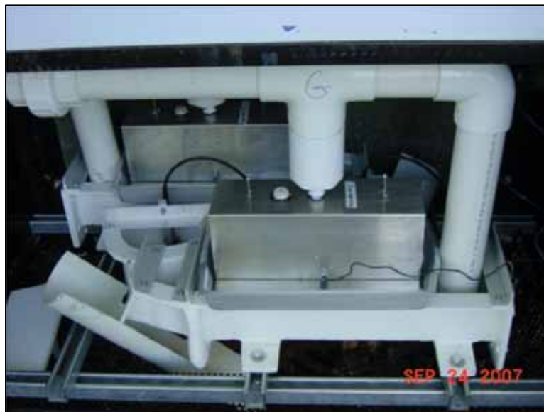
Figure 2-14 Two-Stage Flow Monitoring System (Tipping Bucket Coupled With HS-Flume)
