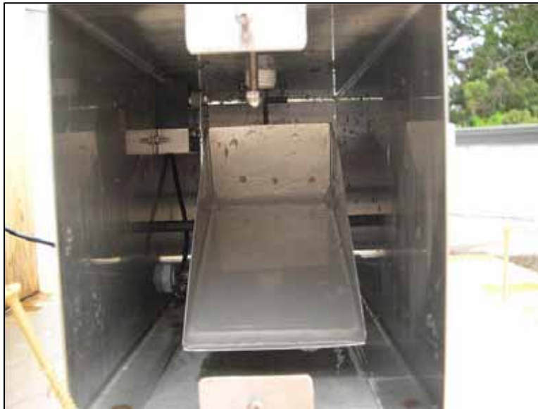
Figure 2-4 Unidata 6506H Tipping Bucket Flow Meter
