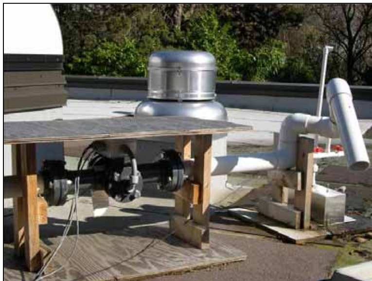
Figure 2-3 Three Inch Unimag DP03ECTERPAA Dual Sensor Electromagnetic Flow Meter
